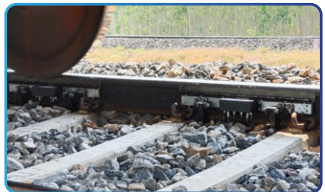
Dual Applicator of 1350 mm long ( 675 x 2 ) can be combined into single or split with the small gap to cover alternate quadrant of wheel
